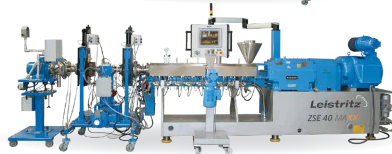
ZSE 40 MAXX with side stuffer, screen changer, gear pump, diverter and underwater pelletizer
