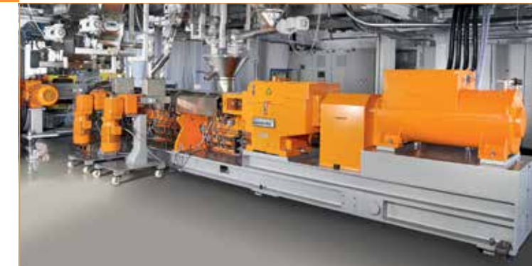
ZSE 75 MAXX high filler loading system with two side stuffers
